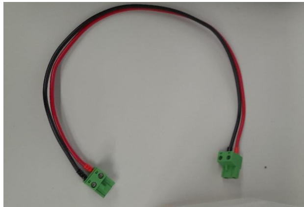
Figure 1. Power distribution cable with crimped ends.
